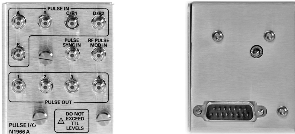
Figure 5. Pulse I/O adapter (N1966A) simplifies connections
